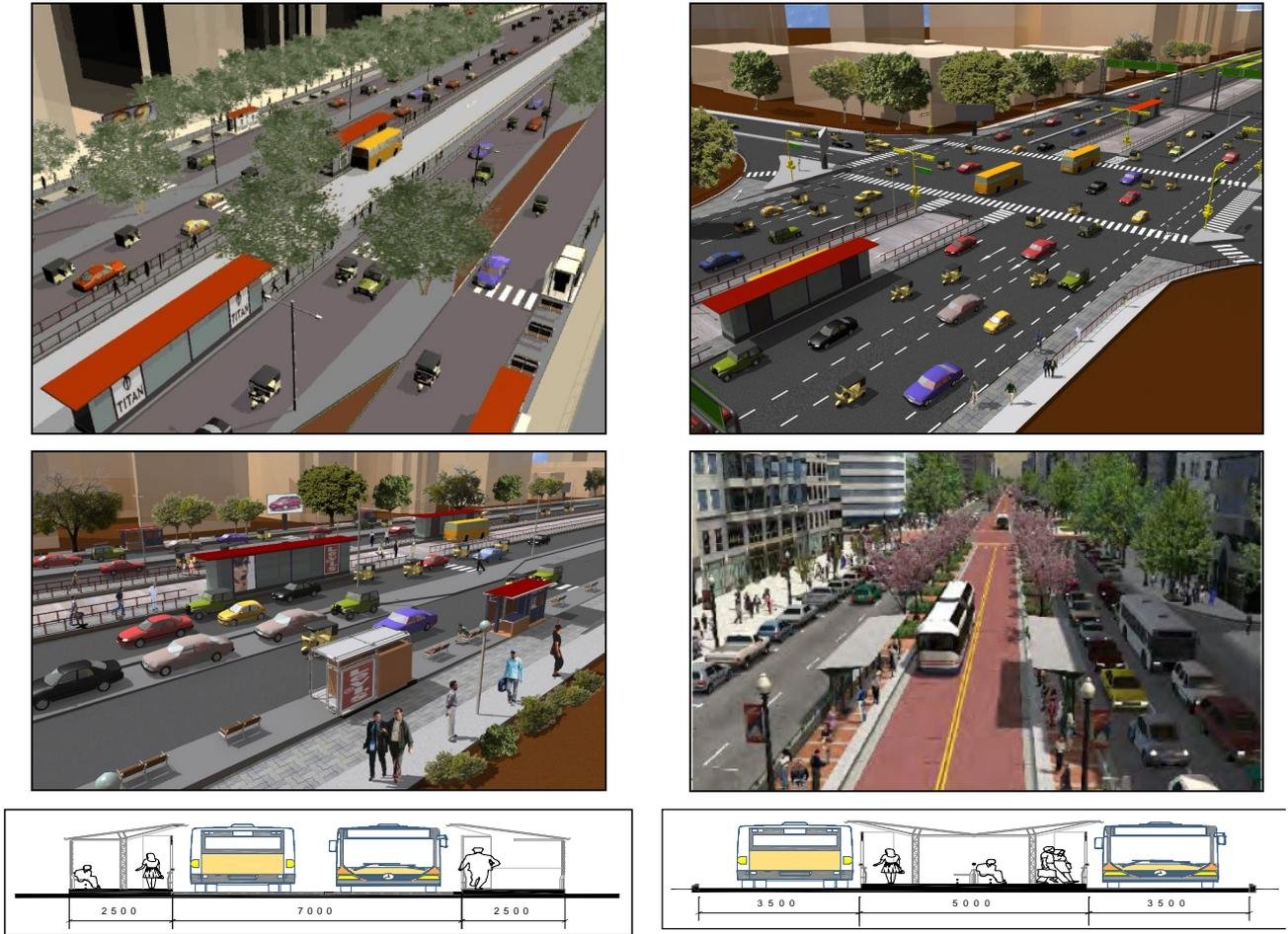
Figure 0-9: Placement of Bus Stops and Junction Treatments
